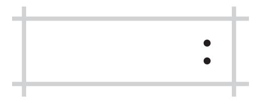
Now make two 10mm holes in the rigid support. Then take two pieces of plastic or rubber pipe with the same external diameter and maximum thickness of 2mm (it's important to leave at least 6mm free), scatter some silicon on the outer part of the pipes end put them in the holes. Cut off the excesses of rubber pipes. The ribbons with the insulating sheath (or all the long wires coming from the module if you have already soldered them to the ribbons) will pass through these pipes.
