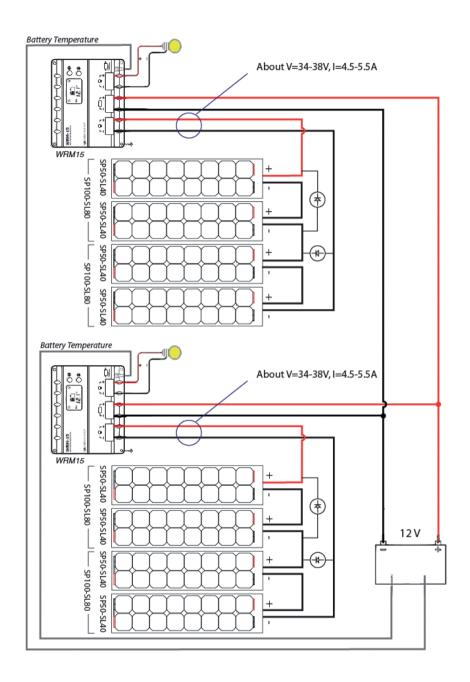
Connecting more modules in series and/or in parallel the voltages and/or the current increase for safety reasons, it is necessary to add some other devices. For example in the following example blocking diodes are inserted to each series of two modules, so to avoid that some of these series becomes a "load" for the other modules when it is under shadow.
