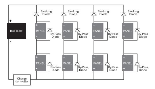
For protection from surges (ex: lightning) it would be worth to use also fuses (one for each string) and isolators to disconnect the strings in the event of failure or maintenance fuses. Of course the choice of the block diodes, fuses, etc.depends on the electrical configuration and must be done by skilled personnel.
